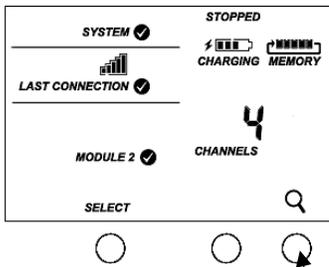
Press this button so the station is ready to have the repeater join the network
