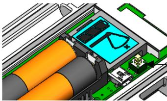
Press this button for 3 seconds for the repeater to join the network
