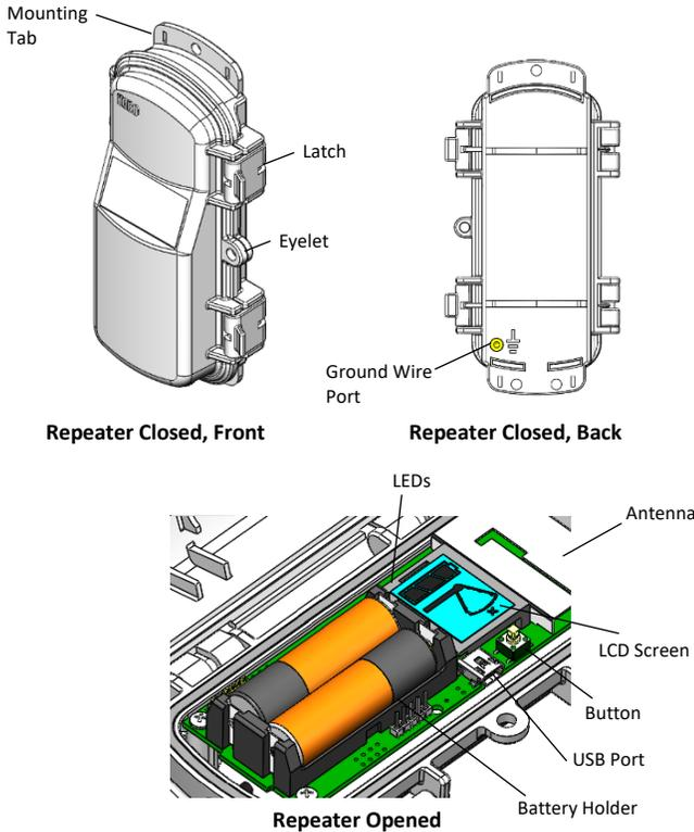
**Mounting Tab:** Use the tabs at the top and bottom of the repeater to mount it (see *Deploying and Mounting*).
