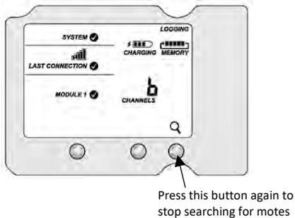
If you added more than one more mote to the network, then the total channel count on the station LCD for the manager module will represent all measurement channels plus a battery channel for each mote in the network.
